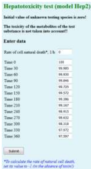
Figure 9. Initial data of material cyto-toxicity (direct toxicity) with fixed degradation rate and calculated results.
